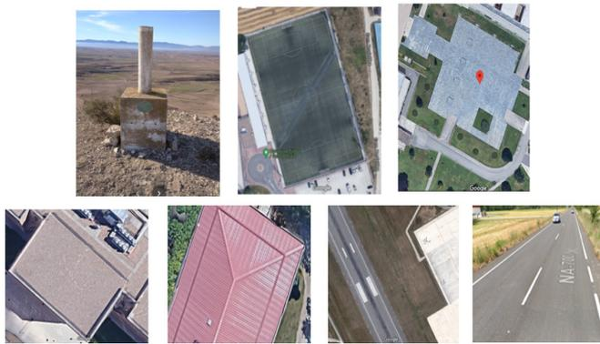
Figure 2. Example of control entities: geodetic monument, football pitch, parking zone, flat roof, pitched roof, airfield runway and a road
